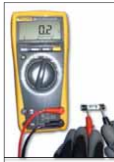
A FUSE WITH THE METER READING "GOOD"
