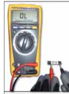
A FUSE WITH THE METER READING "BAD"
