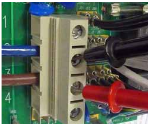
Brown to Blue Wires on a 230V BP2100 System
